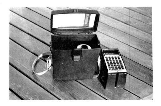
The <u>AccuMeasure</u> is an electronic distance measuring instrument which uses a disposable thread to measure horizontal and vertical distances, angles, and gives 47 more trigonometric, algebraic, and arithmetic functions. Distances can be measured in any Imperial or Metric unit. Angles can be measured in degrees, radians, or grads.
